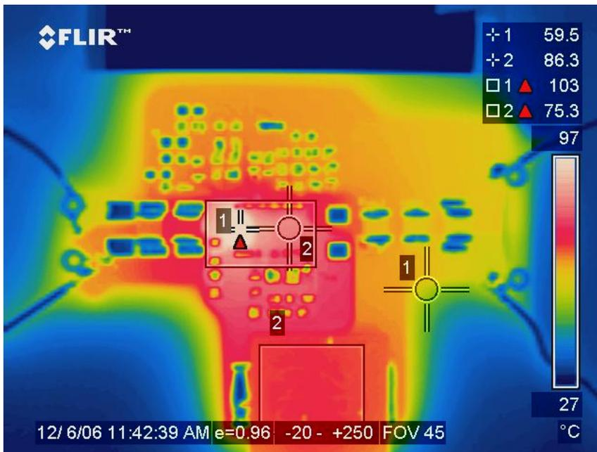
Image 2 – Vin: 12V Iout: 8.0Amps Ambient Temp: 25°C Airflow: 0l/m Pdiss: 3.1W
