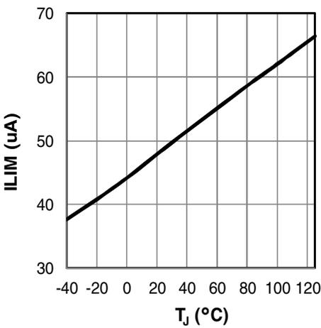
Figure 9:  $I_{LIM}$  versus temperature
