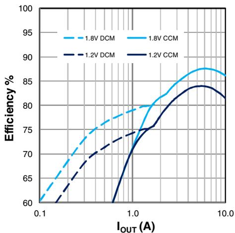
Figure 23: Efficiency,  $V_{IN}=19.6V$
