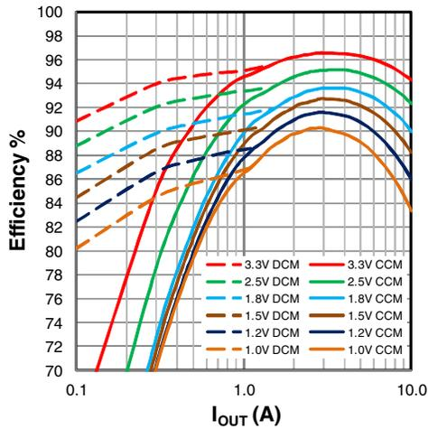
Figure 19: Efficiency,  $V_{IN}=5V$
