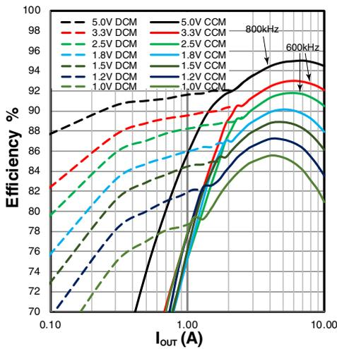
Figure 21: Efficiency,  $V_{IN}=12V$
