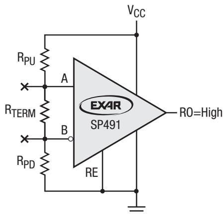
Figure 4: Standard Failsafe with Termination Resistor ( $R_{TERM}$ )
