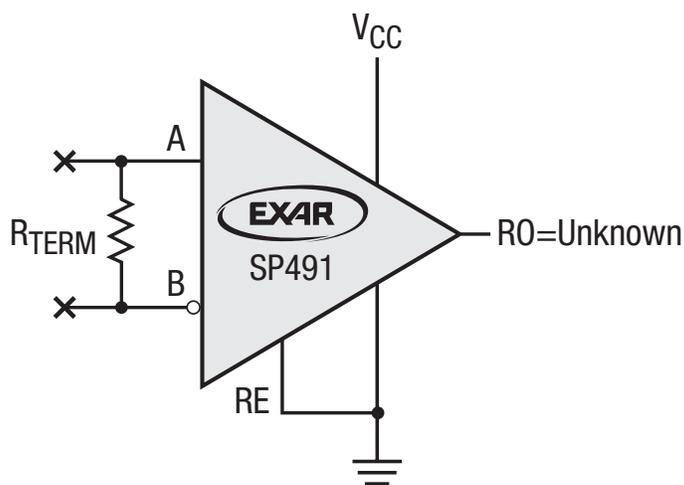
Figure 2: Standard Failsafe with Termination Resistor ( $R_{TERM}$ )
